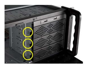
3. Using a flathead screw driver to press the Yellow circle to move the front panel out.
